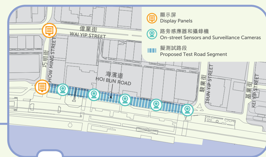
路旁上落貨區監測系統 Kerbside Loading/Unloading Bay Management System
